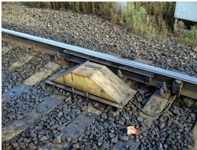
Figure 2 Stationary rail lubricator (SRL-02)
