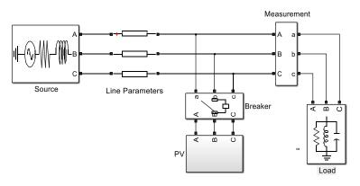
Figure 1 Power system with solar inverter
