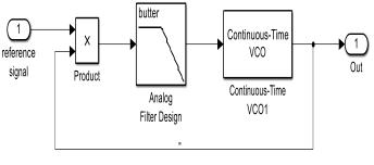
Figure 3 PLL block diagram
