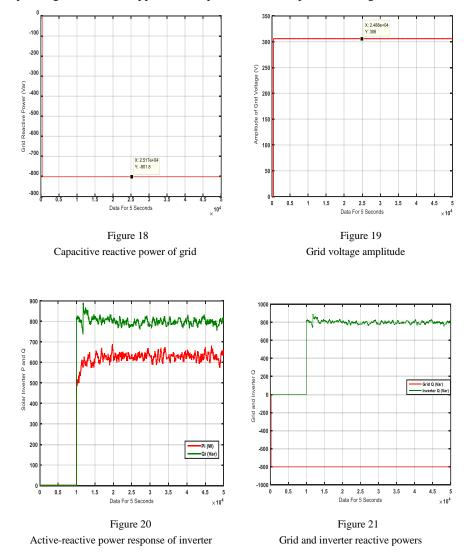
power generation, the remaining power capacity of it is spent on inductive reactive power generation to suppress the capacitive reactive power in the grid.
