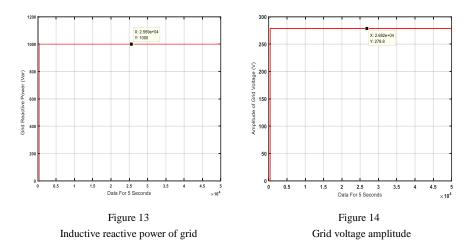
Figure 14 shows that the grid voltage is 278.8 V, which is the critical voltage value due to the active and reactive power supplied by the system. In this case, the response of the inverter in terms of active and reactive power generation was given in Figure 15.
