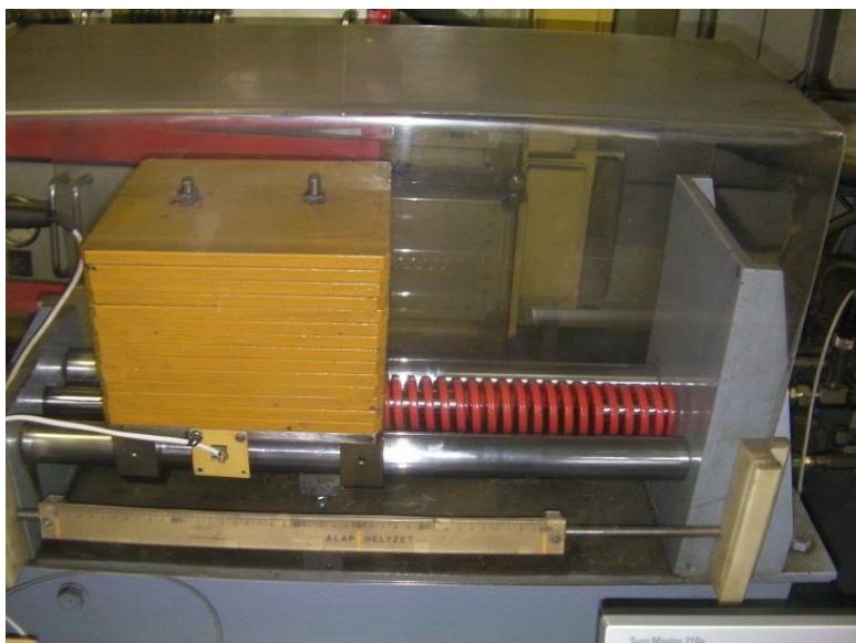
Figure 10 Mass-spring mechanical load of the positioning system
