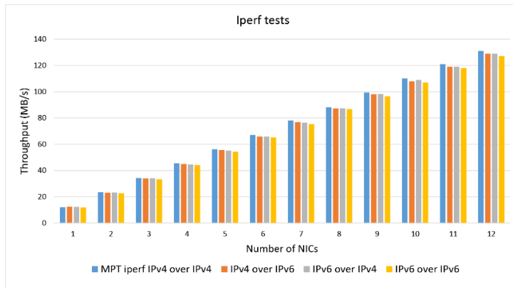
Figure 4 The MPT iperf tests
