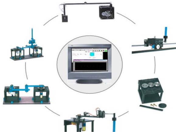
Figure 2 Development system based on different PC controlled electromechanical models
