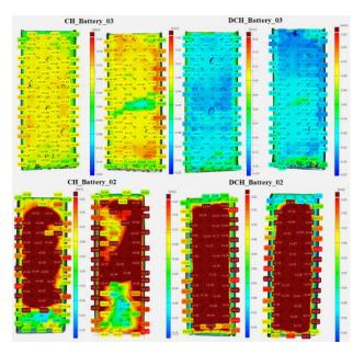
Figure 2 Deformation images recorded using the DIC technique
