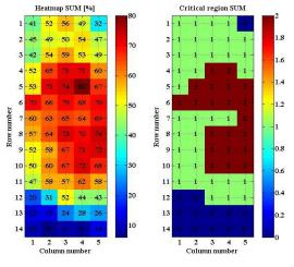
Figure 14 Categorized critical regions of the 5 Ah lithium polymer battery
