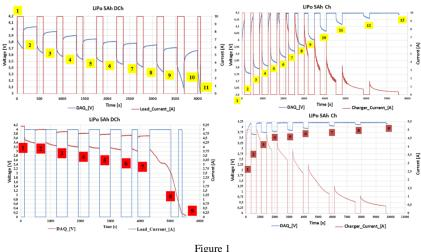
Charging and discharging characteristics of LiPo batteries
