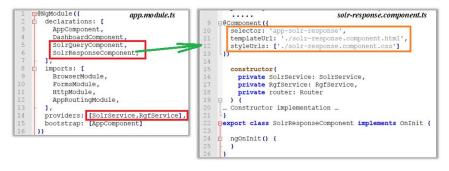
Figure 6 Modular design of Angular application
