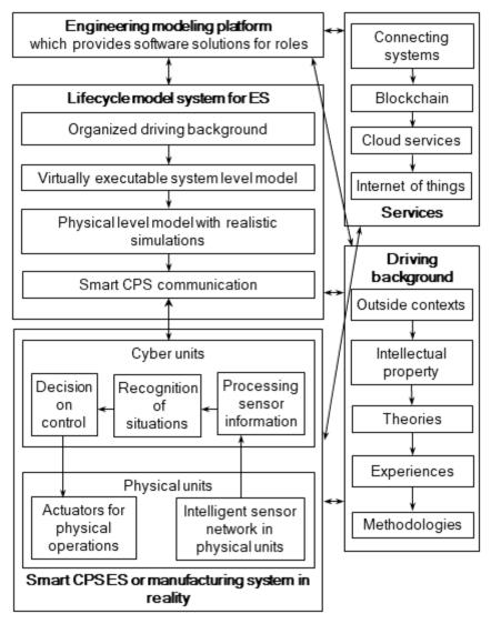
Figure 1 General model of integrated smart engineering system
