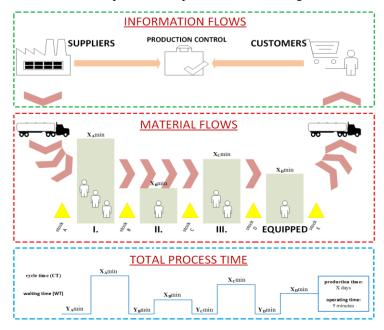
• The bottom of the map is used for process time recording
