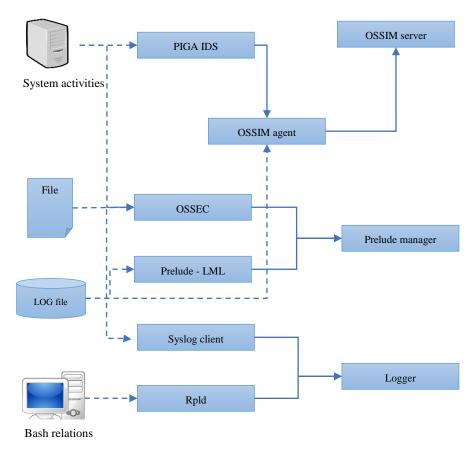
Figure 2 Tools and intrusion detection systems monitoring activity on the hosts
