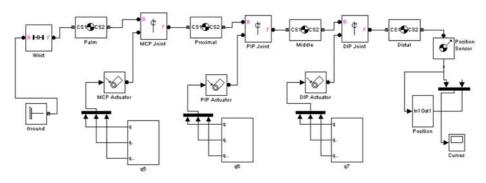
Figure 2 The Simulink model of the middle finger
