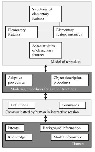
Figure 5 Modeling in recent CAD/CAM systems
