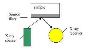
Figure 5 EDX 700 type measuring machine
