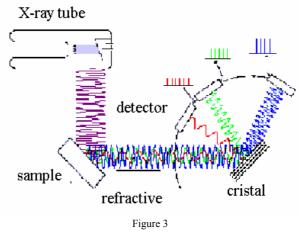
Structure of a wavelength-deflecting spectrometer
