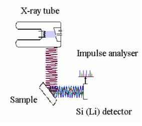
Figure 4 Energy-controlling XRF sprectometer
