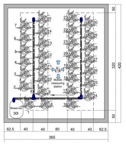
Figure 5. Greenhouse top view with the mobile measuring station
