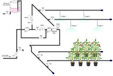
Figure 3. Humidity and irrigation system
