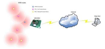
Figure 1. Schematic of the operational sensor network
