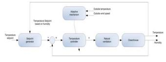
Figure 4. Temperature controller
