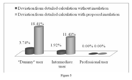
Deviations of calculated heat losses from detailed calculation
