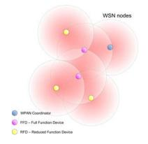
Figure 3. Typical wireless sensor network (WSN)
