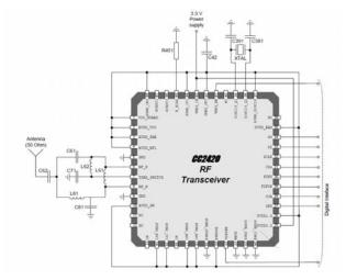
Figure 4. Typical application circuit for CC2420
