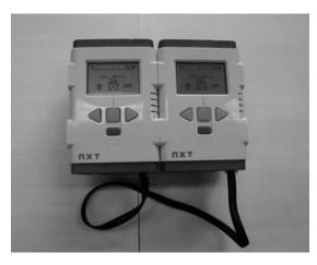
Figure 2 Two NXT central units connected to each other by a sensor cable through their RS485 ports.
