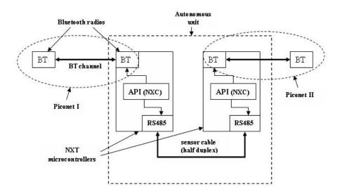
Figure 1 The architecture of the autonomous communication unit consisting of two NXT microcontrollers.
