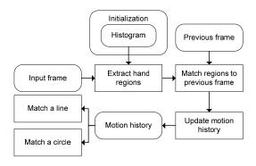
Figure 3 Block diagram of the hand tracking and movement estimation
