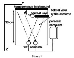
The experimental setup (d is the distance of the tip of the index finger from the homogeneous background)
