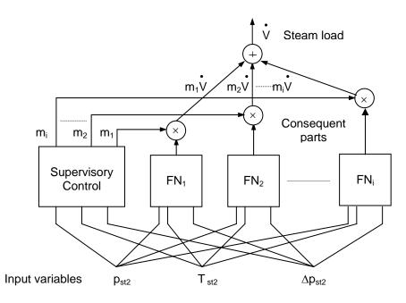
Figure 2.11. Scheme of supervisor system for the heat power station
