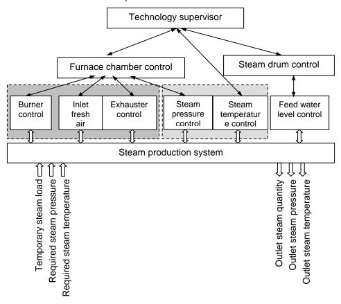
Figure 2.1. Hierarchical control strategy for the large-scale system of steam production
