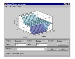
Figure 2.6. Fuzzy control for setting the fuel valve by Sugeno's rule
