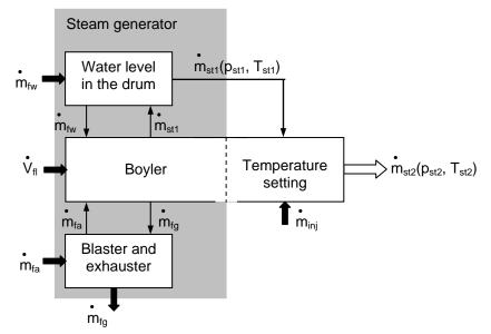
Figure 2.2. Controlled parameters of steam production technology
