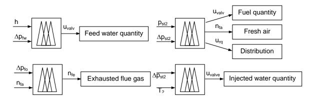
Figure 2.3. Structure of FISs for the control of steam production system
